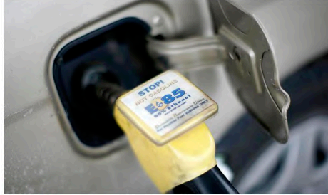
Smooth transition: E85 is a fuel blend made of up to 85% ethanol and 15% petrol (gasoline) REUTERS
